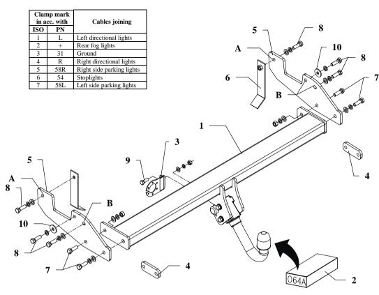
This towbar is designed to assembly in following cars: **TOYOTA HILUX 4WD with double cabin,** produced since 10.2005 till 10.2010, catalogue number **064A** and is prepared to tow trailers max total weight up to **2500 kg** and max vertical load **100 kg**.
