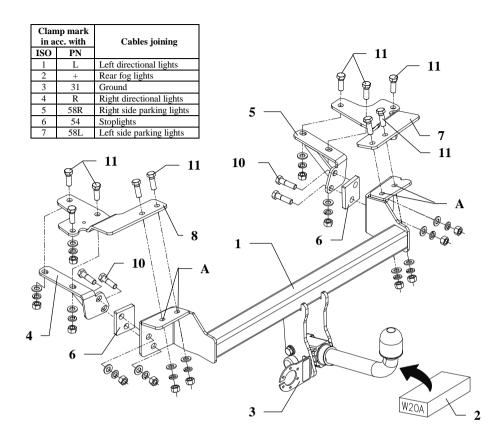
This towbar is designed to assembly in following car: **SUZUKI LIANA, 4 doors,** produced since 03.2002 till 12.2007, cat. no. **W20A** and is prepared to tow trailers max total weight **1200 kg** and max vertical load **75kg**.
