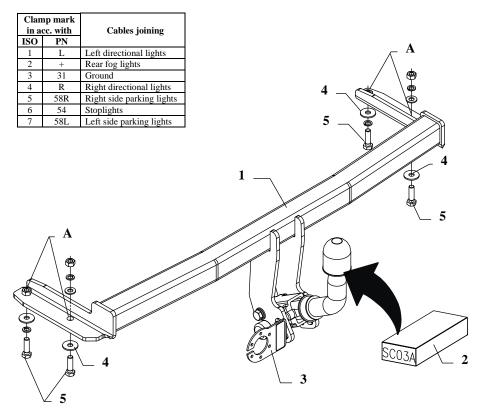
This towing hitch is designed to assembly in following cars: **SEAT IBIZA, 3/5 doors (6K),** produced since 10.1999 till 03.2002, catalogue no. **SC03A** and is prepared to tow trailers max total weight **1100** kg and max vertical load **50 kg**.
