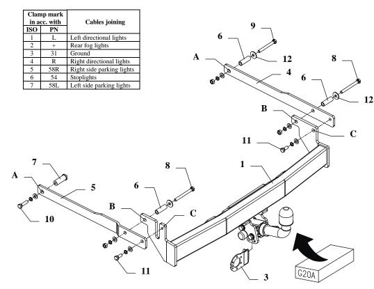
This towing hitch is designed to assembly in following cars: **RENAULT SAFRANE, 5 doors,** produced since 04.1992 till 12.2001, catalogue no. **G20A** and is prepared to tow trailers max total weight **1600 kg** and max vertical mass **75 kg**.
