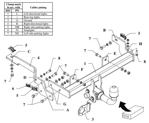
This towing hitch is designed to assembly in following cars: **PEUGEOT 106, 3/5 doors,** produced since 05.1996 till 07.2003, catalogue no. **F01A** and is prepared to tow trailers max total weight **1100 kg** and max vertical load **50 kg**.
