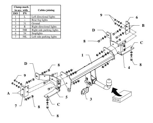
This towing hitch is designed to assembly in following cars: **OPEL ANTARA (C105)**, produced since 11.2006 till 05.2011 and since 06.2011, catalogue number **E51A** and is prepared to tow trailers max total weight up to **2000 kg** and max vertical mass **80 kg**.
