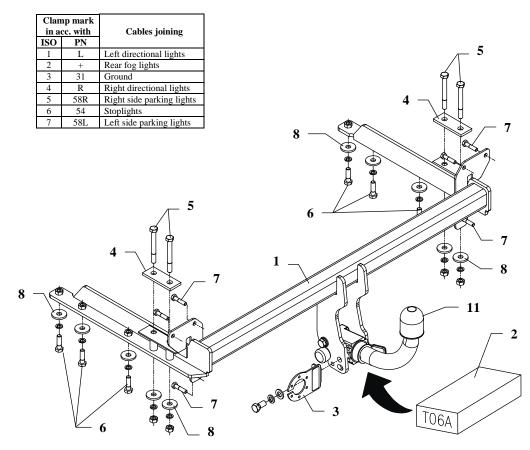
This towbar is designed to assembly in following cars: **KIA SEPHIA II, 4 doors, KIA SHUMA II, 5 doors (FB),** produced since 10.1997 till 12.2004, catalogue no. **T06A** and is prepared to tow trailers max total weight **1350 kg** and max vertical load **50 kg**.
