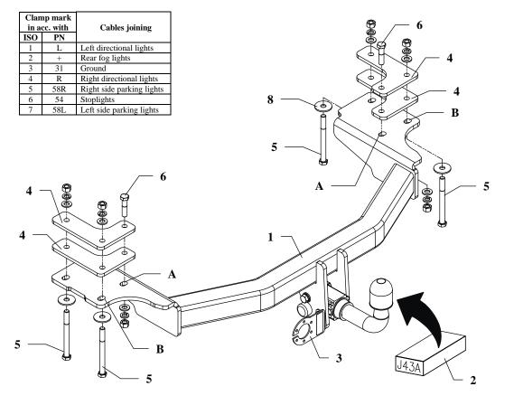
This towing hitch is designed to assembly in following cars: **HYUNDAI TERRACAN HP1**, produced since 12.2001 till 01.2007, catalogue no. **J43A** and is prepared to tow trailers max total weight **2800 kg** and max vertical mass **115 kg**.
