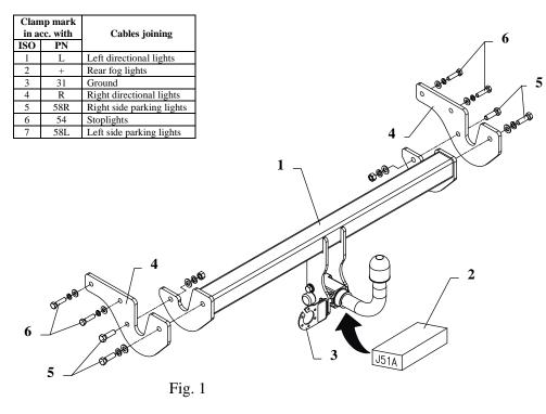
This towing hitch is designed to assembly in following cars: HYUNDAI SONATA 4 doors (NF), except V6, produced since 03.2005, catalogue no. J51A and is prepared to tow trailers max total weight 1700 kg and max vertical load 75 kg.
