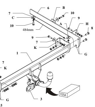
This towing hitch is designed to assembly in following cars: **HONDA CIVIC AERODECK ESTATE**, produced since 1997 till 02.2001, catalogue no. **Y05A** and is prepared to tow trailers max total weight up to **1300 kg** and max vertical mass **50 kg**.
