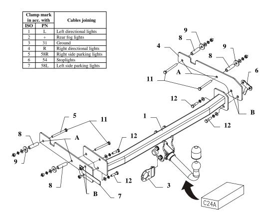
This towing hitch is designed to assembly in following cars: **FORD FIESTA COURIER delivery van (J3S, J5S)**, produced since 02.1996 till 12.2002, catalogue no. **C24A** and is prepared to tow trailers max total weight **900 kg** and max vertical load **50 kg**.
