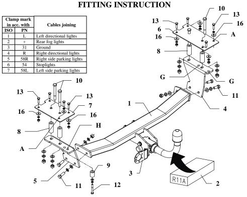
This towing hitch is designed to assembly in following cars: **FIAT MAREA 4 doors** (185), produced since 10.1996 till 10.2001, catalogue no. **R11A** and is prepared to tow trailers max total weight 1400 kg and max vertical load 70 kg. *Before installation look at the page 337 in the instruction of the car*.
